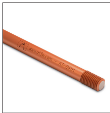
AT-041H Pica ø16 x 2000mm rosca 5/8" cobrizada 254µm
