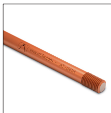
AT-041H Pica ø16 x 2000mm rosca 5/8" cobrizada 254µm
