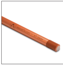
AT-041H Pica \varnothing 16 x 2000mm rosca 5/8" cobrizada 254 \mu m
